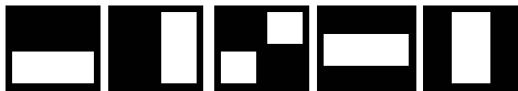
Figure 2. Candidate filter set. We select a compact set of filters from the filter class employed for object detection by Viola and Jones. When applied to spectrogram images, these filters capture important time-frequency characteristics of audio.
